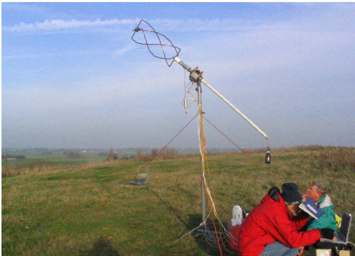
Fig. 6. The RQHA-12 under test (notice the weight to balance the set-up)
